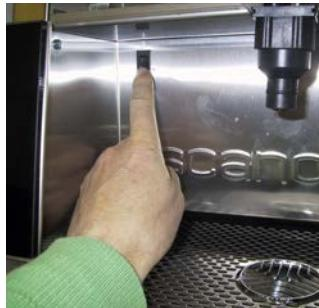
Sluk for maskinen
