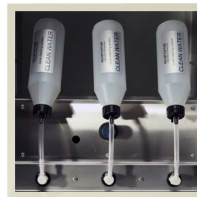
6. Connect the bottles with the blue writing, which should contain cold clean water, and press "Clean" again.
