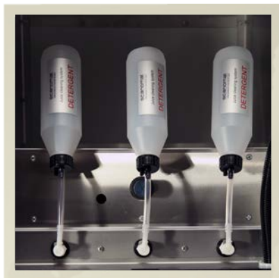
4. The plastic bottles with warm water with the cleaning tablet should be connected. Open for the flow by turning the valve so that it is horizontal to the tube.
