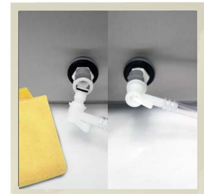
3. Always be aware that the connecting parts are clean and if not, clean with a warm damp clothe.
