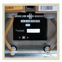
7. When the procedure is finish remove the bottles and reconnect the juice boxes to the unit. Once done, make on of each drink to ensure that the concentrate is pumped to the mixing system.
