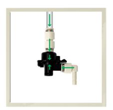
7. All parts are reassembled, please be ensure that the tubes are fully inserted into the connectors.
